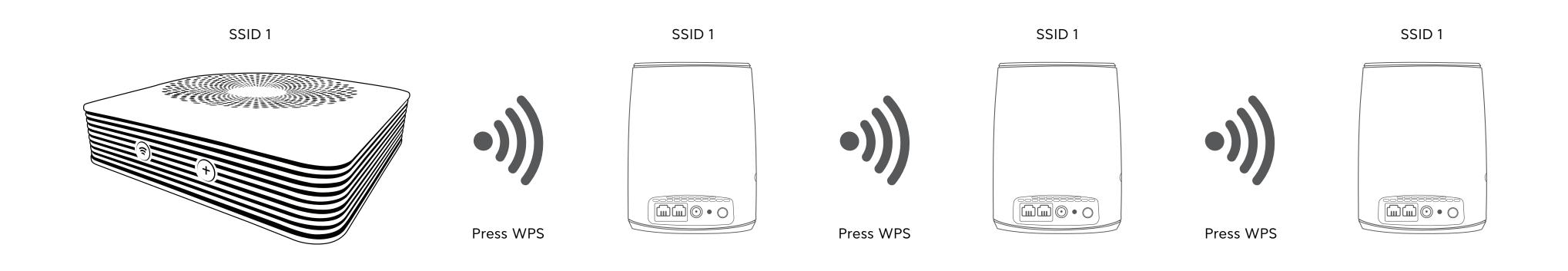
Note: The Wi-Fi Name / SSID and Wi-Fi Password of the Wi-Fi Pod will be cloned from the modem.
